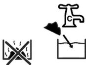
In situations of excessive shear heat place purgings in cool water to eliminate fumes
