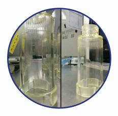
2 rejects; both with one black spec and the first with splash marks (no back pressure)
