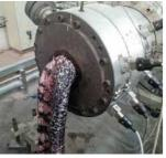
Pipe extrusion – with its demanding materials and even more demanding die designs and sizes – has always been an enigma to manufacturers of purging compound. Designing something that effectively and eff ciently clears PE100 from a 600mm basket die is too much for your average R&D team. On top of that, PE80 is highly unlikely to clear out their purging compound.
