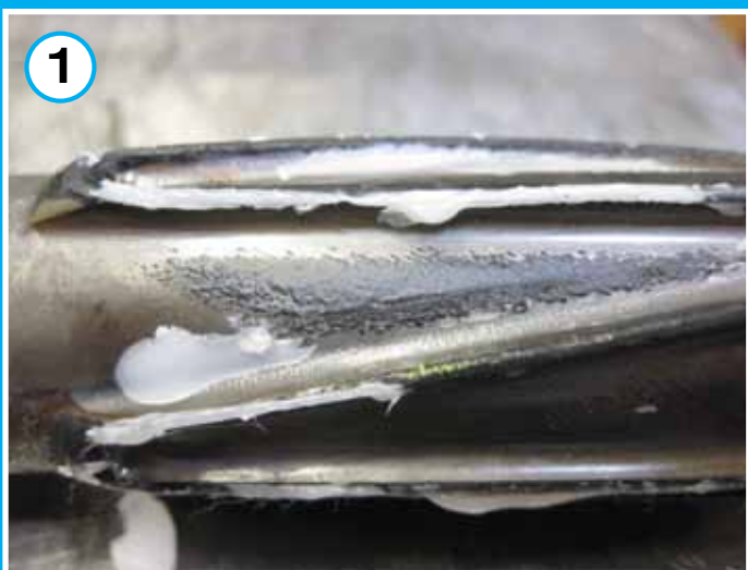
Mixing section of POM Ø30mm screw extracted for photo and replaced "uncleaned"
