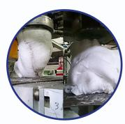
By the end of 100 kg the majority of the carbon was gone (Left). Last full stroke shows no more residue of carbon/colour (Right). Machine is switched off for ddecarbonisation
