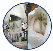
The photos show the build-up of carbon on the inside being removed by the decarbonising, on set up on Monday morning
