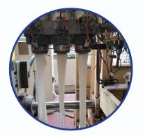
PolyClear HMEX works in the low compression areas of the head, as a result the colour lines are gone and next production can start.
