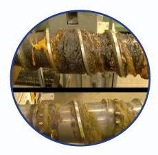
Material supplier issue caused massive degradation
