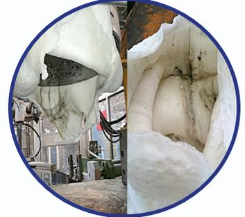
The photos show the build-up of carbon on the inside being removed by the decarbonising, on set up on Monday morning
